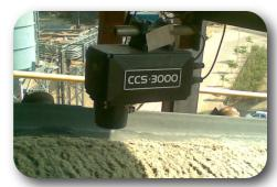
Moisture measurement and control is a crucial aspect in coal processing. MoistTech's new CCS3000 Moisture Sensor provides the user with non contact instant moisture measurement.
