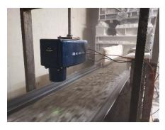
Measuring and controlling moisture can reduce transportation costs due to shipping excess water. Additionally, moisture control stops products from freezing during shipping and transportation.
